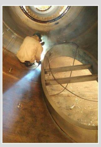
In the manufacturing process of wind power barrel, in the position of the welding joint or the heataffected zone of the door frame is prone to be caused with slightly fining cracks after welding, and the thicker the steel plate to the greater the tendency of cracks. The welding stress, temperature, process, and hydrogen gathering are the main reasons, and whereas, the solutions are herein, including the welding materials.
